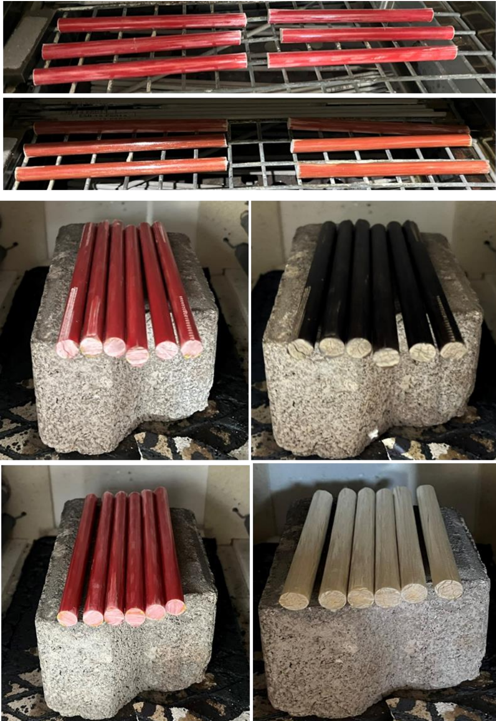
Fig. 3. GFRP bar specimens before and after exposure to thermal load for 200-300 and 500 degrees
