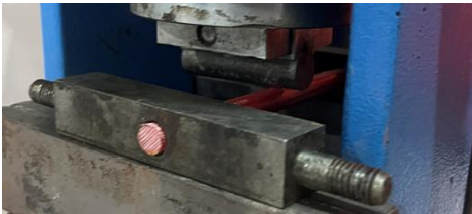
Fig. 2. Experimental Three Point Bending test setup of cylindrical GFRP bar specimen
