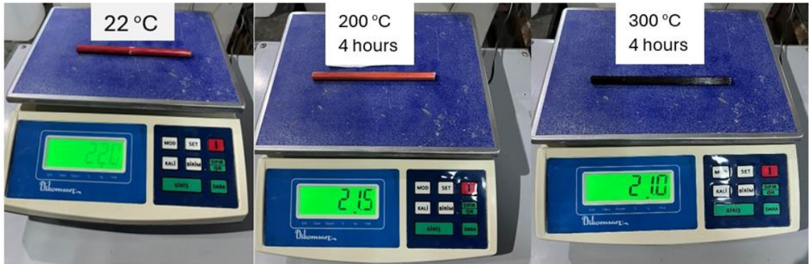
Fig. 8. Examples of weighing GFRP bar samples with precision scales from 22 degrees to 300 degrees
