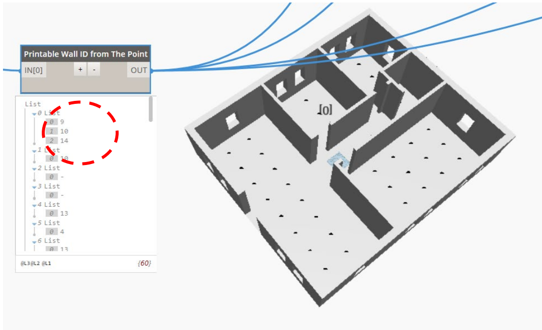
Fig. 6. Example: “Printable Wall ID from The Point” script at Point 0 for Walls 9, 10, and 14
